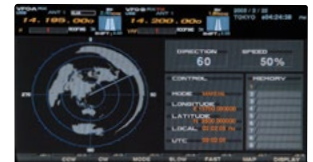
■ Antenna Bearing Indication using Great Circle Map
